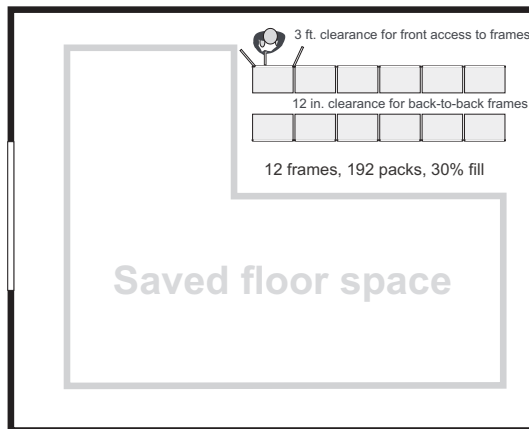
Interfacing 48,000 trunks to the DMS system with Spectrum Peripheral Modules...
