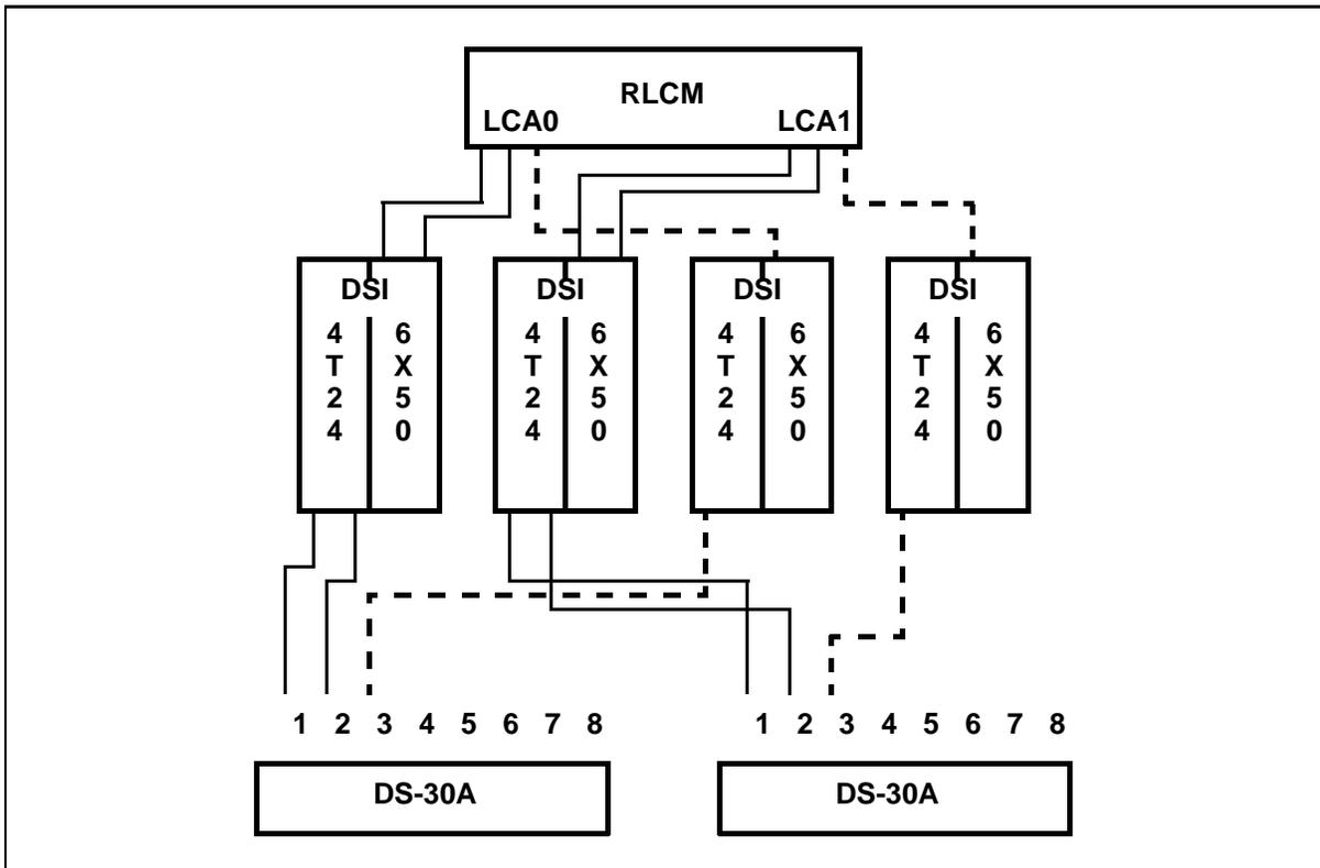
Figure 2-28: Six-loop interface with an RLCM using six DSI modules
