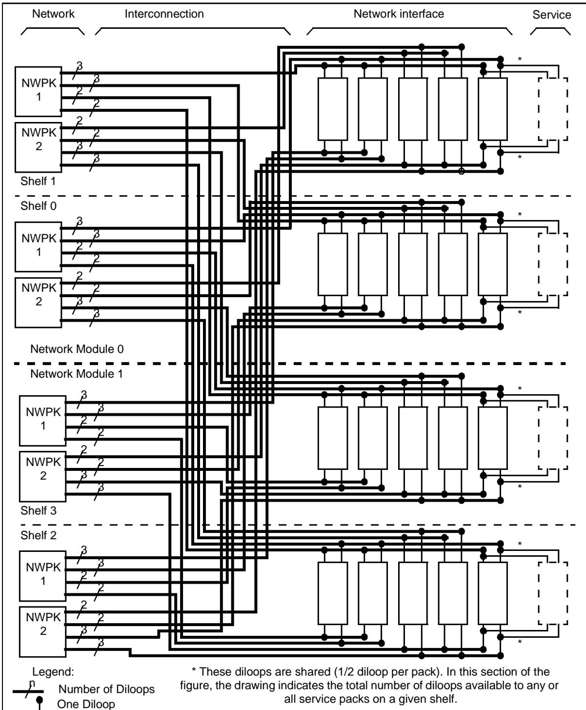
The three-bay configuration consists of one network module (that is, two CPU/Network shelves). Each CPU/Network shelf houses two interface packs (one MLI and one DS-30A) and up to four service packs. Hence, the total loop capacity per CPU/Network shelf is 16 multiplex loops and 8 diloops, or 32 multiplex loops and 16 diloops per network module.
