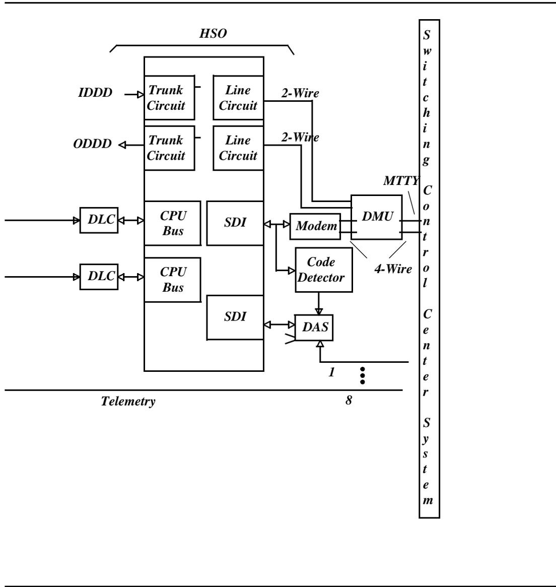
Figure 4-9: Digital link interface between DMS-10 cluster and Switching Control Center System
