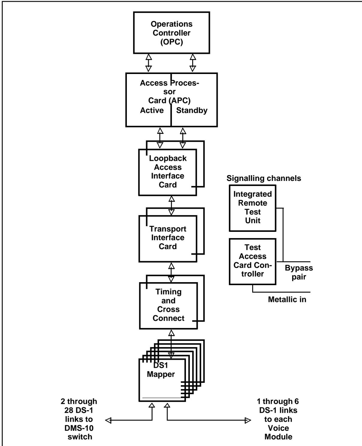
**Operations Controller** The operations controller (OPC) provides operating company personnel interface to the AccessNode for maintenance and administration purposes.
