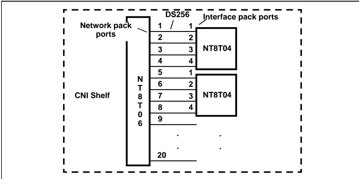
Each DS256 loop is mapped to a specific set of peripheral loops on an NT8T04 pack. If GTSB is not activated on an NT8T04, each of the four DS256 loops is mapped to a group of eight peripheral loops (PELP). If GTSB is activated on an NT8T04, three of the DS256 loops are each mapped to a group of eight peripheral loops and the remaining DS256 loop is split across a set of four peripheral loops and the GTS, as shown in Figure 2-13.
