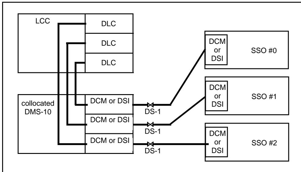
When installed, the collocated DMS-10 switch must be within 50 feet of the LCC. In this arrangement, DS-1 (T-1) spans running from the SSOs can terminate at DCMs or DSIs in the collocated DMS-10 switch.
