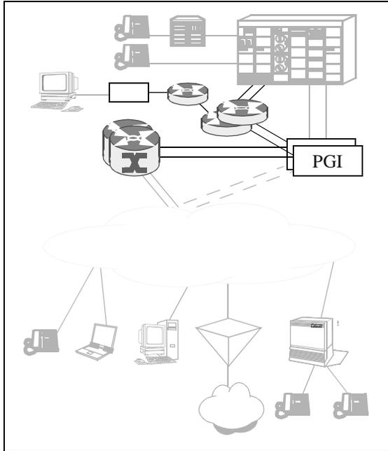
This section describes the data networking equipment and characteristics that comprise the DMS-10 Central Office Local Area Network (CO LAN) in the DMS-10 packet network product offering, as emphasized in Figure 2-51. The main DMS-10 sub-components covered in this section are:
