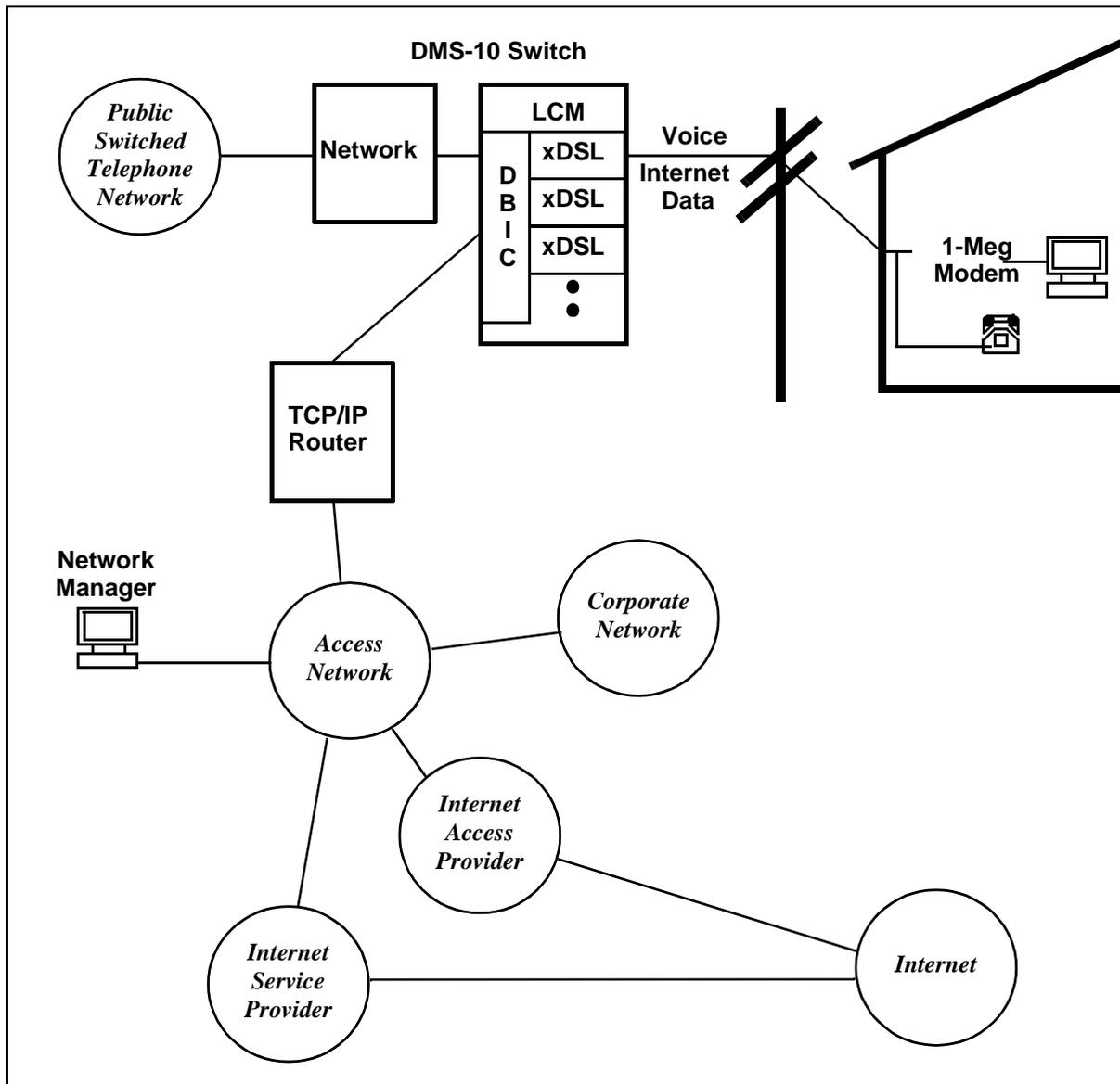
**1-Meg modem** The 1-Meg modem is located at the customer's premises and connects to the customer's telephone line, extension telephone, and personal computer. This modem provides 10Base-T/100Base-T interface rather than a serial RS232 interface. To the subscriber, this modem appears to operate as a regular voice-band modem.
