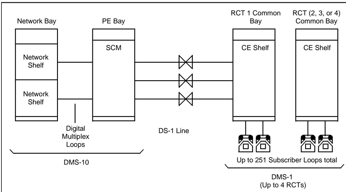
Figure 2-22: SCM block diagram
