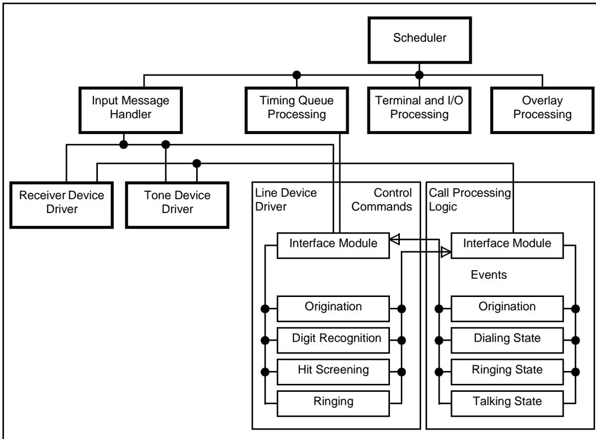
The DS-30A pack or Network Interface pack passes the message to the CPU as an interrupt. The CPU firmware interrupt handler reads the message from the interface pack and puts it in the CPU input message buffer. The input message handler then removes the message from the buffer for processing.
