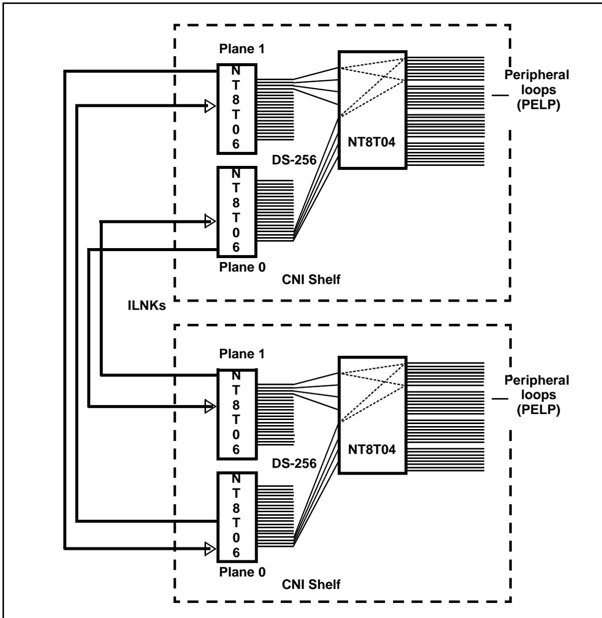
The channels on the DS-256 loop are in fixed relationship to the channels on the peripheral loops. After a peripheral timeslot for the source terminal and the destination terminal is determined to be available, the network connection between the terminals is guaranteed. Thus, network blocking will not occur.
