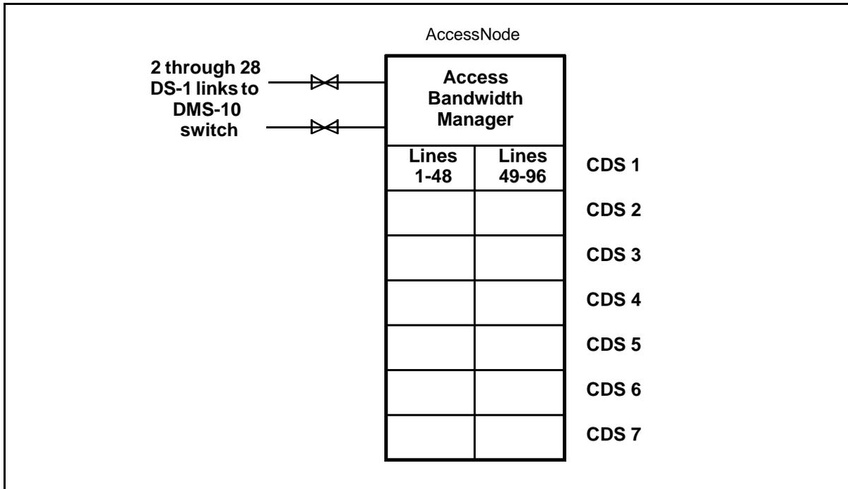
**Access Bandwidth Manager (ABM)** The Access Bandwidth Manager (ABM) provides DS0 switching between the host (DMS-10) DS-1 links and the links to the Narrowband Line Interface cards in the standard AccessNode Copper Distribution Shelf (CDS) drawers. The components of the ABM are shown in Figure 2-32.
