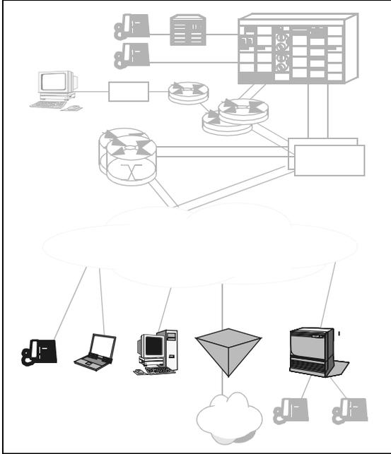
This section describes the IP-based endpoint devices in the DMS-10 packet network product offering, as emphasized in Figure 2-48. IP-based endpoint devices are external to the DMS-10 system and are described here in general terms.
