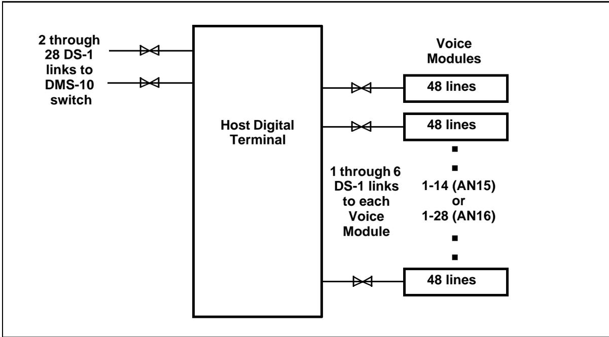
**Voice Module (VM)** A Voice Module (VM) consists of from 1 through 6 DS-1 links, a processor, matrix cards, an Integrated Test Unit (ITU), and up to 48 line cards. Each VM can be configured with a maximum of six DS-1 links.
