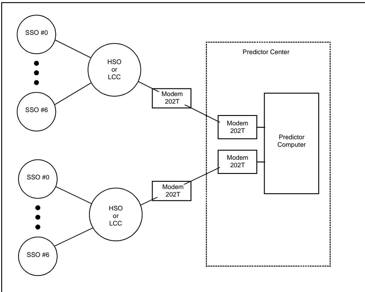
In a cluster configuration with LIT, the HSO or LCC should have only one dedicated output class and one dialup LIT output class for backup. The SSO should have one dialup as backup.
