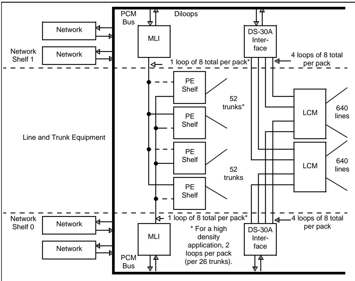
**DS-30A Interface (DS-30A)** DS-30A packs provide an interface between the network and the LCE and SCE. Each DS-30A provides eight DS-30A peripheral multiplex loops, and interfaces them with two or four Network diloops. Each loop is paired with another; one provides 32 timeslots for speech transmission while the other provides 30 timeslots for speech transmission, one timeslot for signaling, and one timeslot unused. Four or six DS-30A loops are provisioned for each 640-line LCM.
